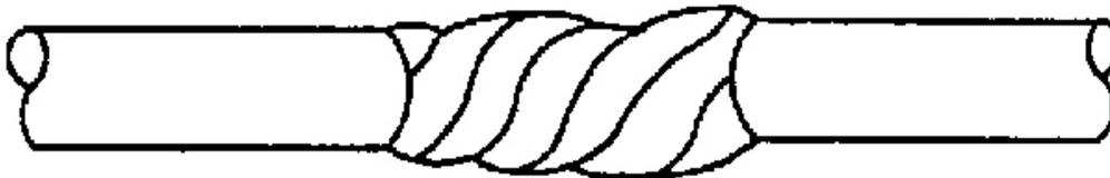
**Fig. 14: Repaired Wire Covered With Electrical Tape Terminal Identification**
